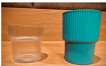
Drinking cup made of polycarbonate. Left: without polymeric additive, right: with polymeric additive from Polytives GmbH, Rudolstadt.
